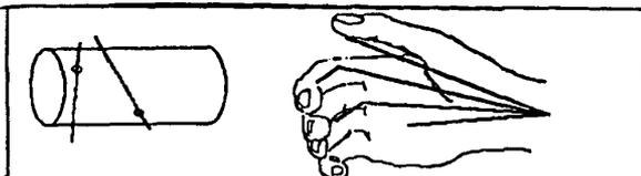
Figure 5: Graphic simulation showing object, task features, and hand parameters. A cylinder is to be lifted, using two oppositions, shown by the two opposition vectors. The two oppositions are seen in the posture taken on by the hand.
