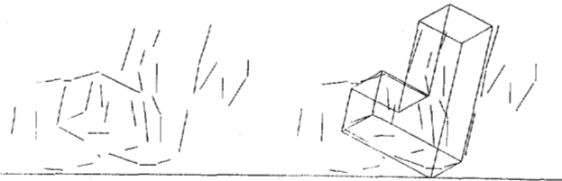
Figure 4. (a) The x, y projection of edge fragments obtained by running the Canny edge detector on a depth map. (b) The projected object model located by the edge matcher superimposed on the edge fragments. This example corresponds to Figure 1.
